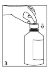
Insert adaptor into the neck of the bottle until a tight seal is made.
