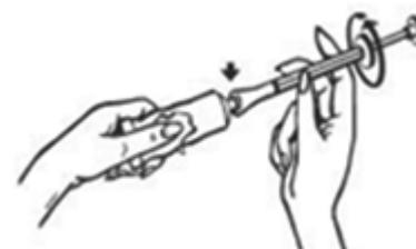
3. Squeeze the tube slowly to fill the applicator to the ring-mark (where the plunger stops).
