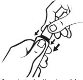
2. twist in the direction of the arrow as shown below (counterclockwise).
