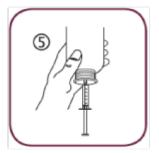
Fill the syringe with a small amount of solution by pulling the piston down (5A), then push the piston upward in order to remove any possible bubble (5B). Pull the piston down to the graduation mark corresponding to the quantity in milliliters (mL) prescribed by your doctor (5C)
