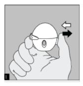
To release the dust cap press the piercing button completely in and let go.
