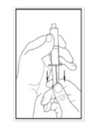
9. Attach the syringe to the clear end of the transfer device by turning it clockwise.
