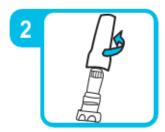
Just before use, remove the Podhaler device from its case by holding the base and twisting off the top of the case in a counter-clockwise direction. Set the top of the case aside. Briefly inspect the inhaler to make sure it is not damaged or dirty, and then stand it in the base of the case.
